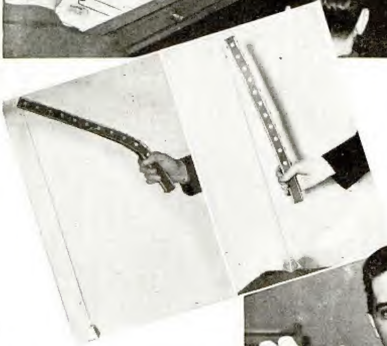
Above, jointed flexible model of the human spine shows why heavy load should be lifted with the legs and not the back, which is easily strained if legs are not properly used. The picture at left illustrates the wrong system with the model spine bending. When strain is taken with "legs" (right) the spine remains straight
